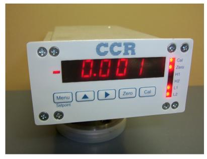
The Model SR5 can be mounted in a panel cutout or simply used as a bench-top instrument. It is packaged in a small 1/8 DIN, 5.5" deep extruded aluminum housing which provides excellent EMI/RFI shielding and good heat dissipation characteristics. The transducer is connected to the 15-pin type-D standard electrical connector and accessory signals are accessed via the 15-pin type-D high density electrical connector.
