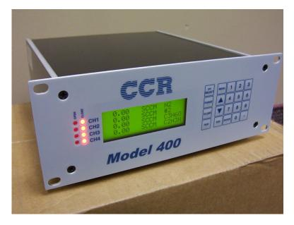
The Model 400 can be rack mounted or simply used as a bench-top instrument. It is packaged in a standard half-rack housing which provides excellent EMI/RFI shielding and good heat dissipation characteristics. The transducers are connected to the 15-pin type-D standard electrical connector and accessory signals are accessed via other electrical connectors at the rear of the instrument.
