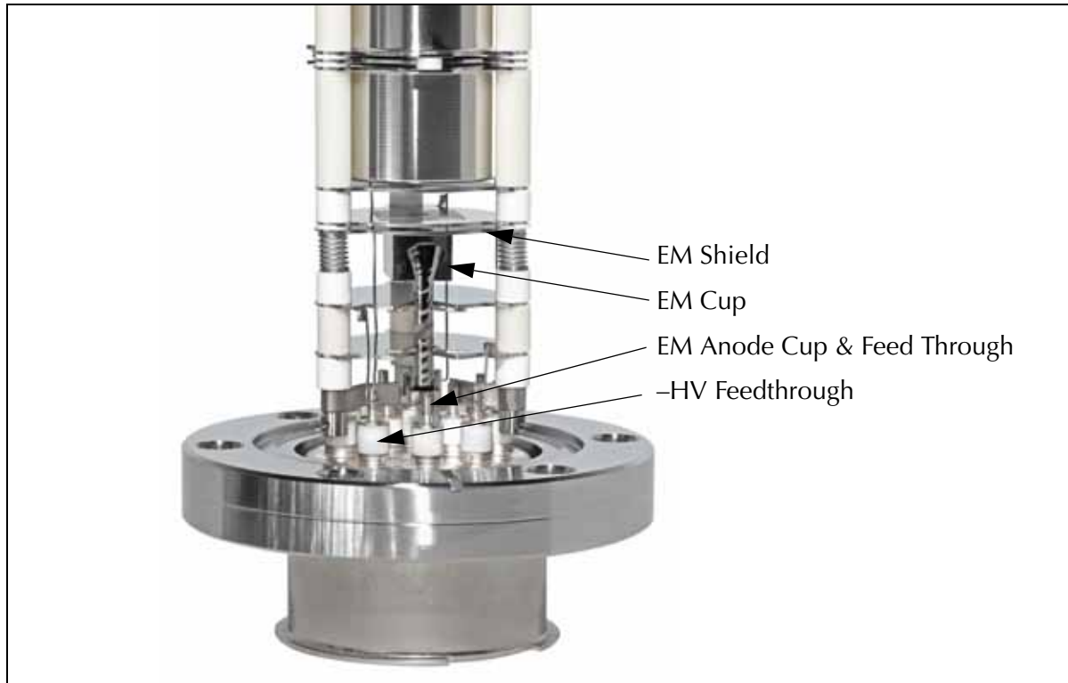
Figure 6-6 MS Gauge Electron Multiplier Assembly
