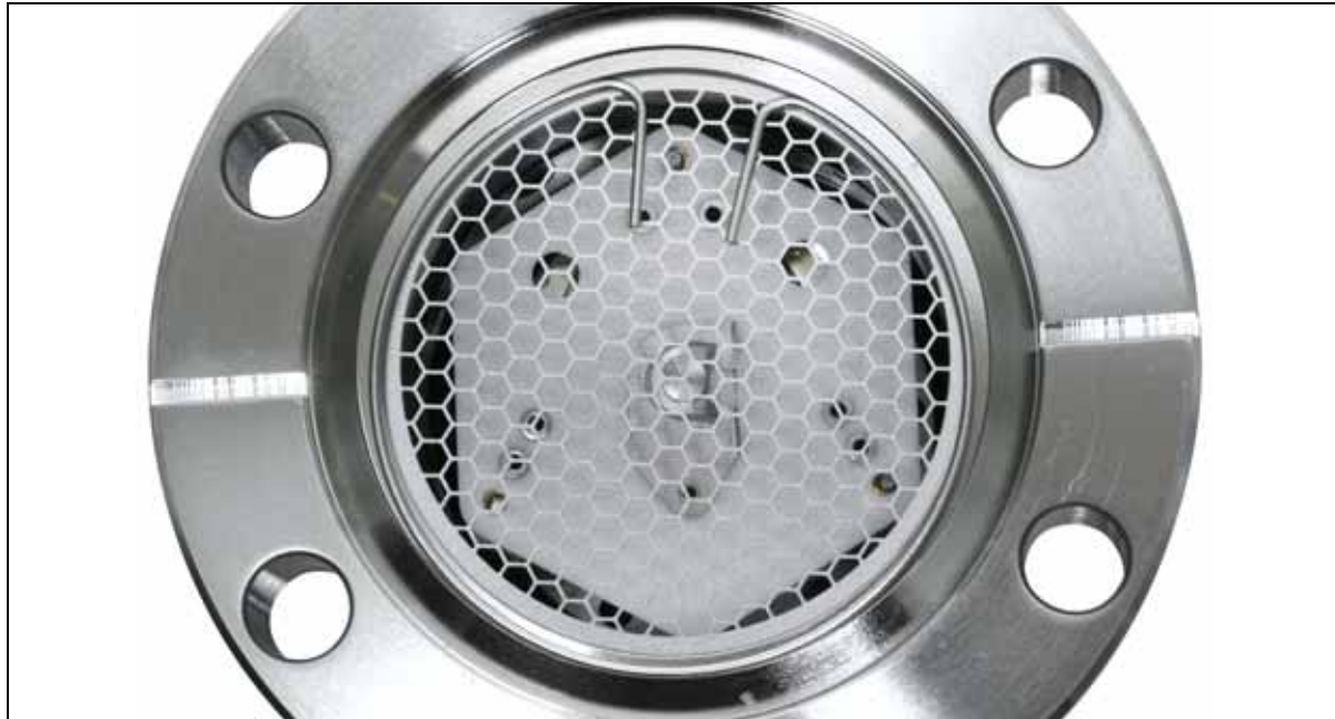
Figure 6-8 Plasma Screen in the Demountable Envelope (4-inch Nipple)
