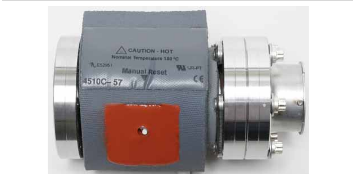
Figure 3-5 Optional Heater Jacket on a VQM MS Gauge
