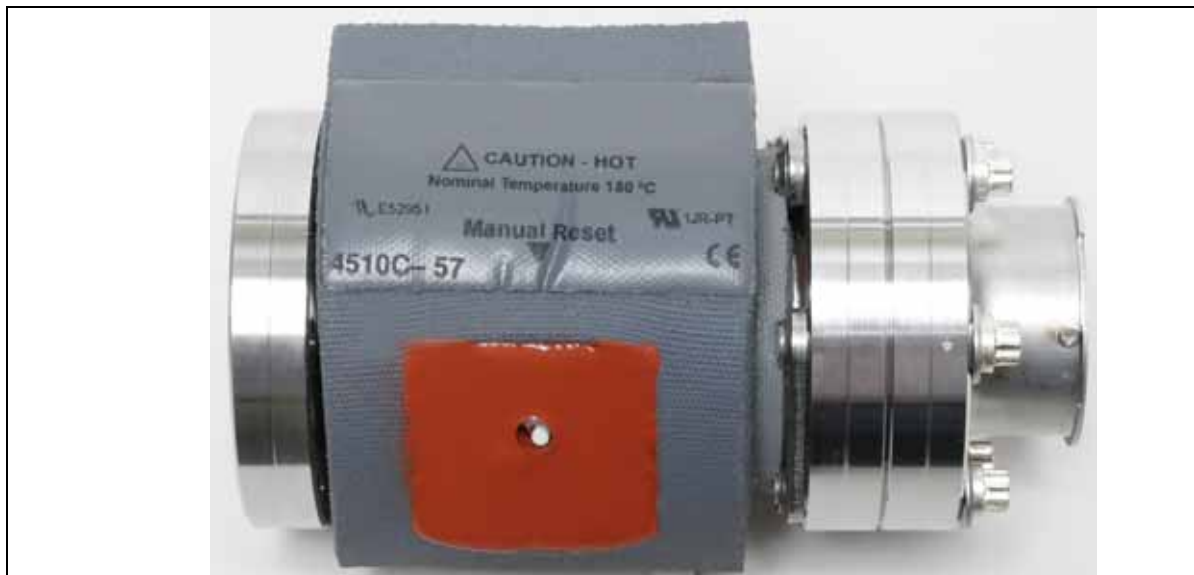
Figure 6-7 MS Gauge with Heater Jacket
