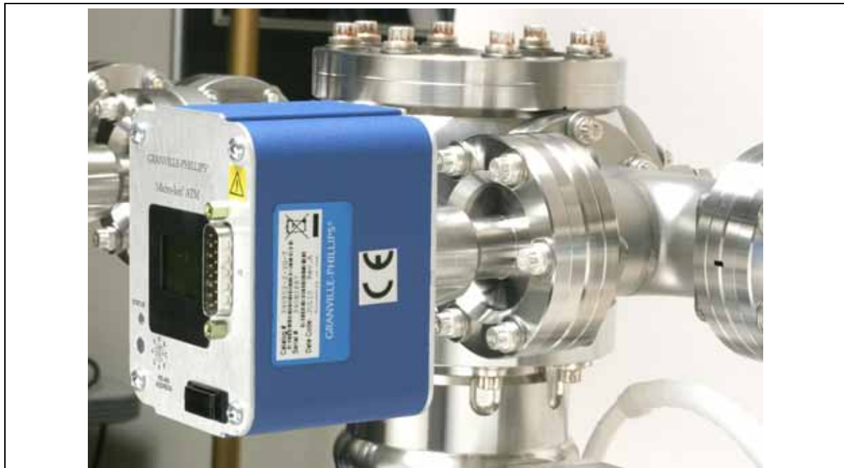
Figure 3-6 Micro-Ion Gauge Mounted on a Vacuum Chamber
