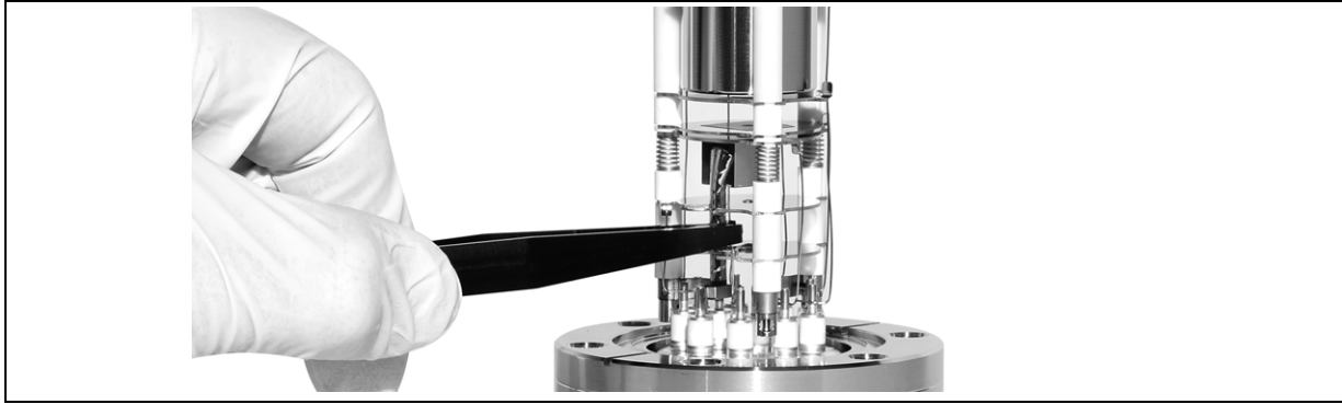
Figure 7-11 Remove the Electron Multiplier
