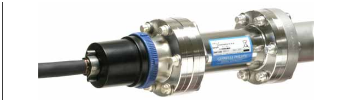
Figure 3-8 Cable Connected to the MS Gauge
