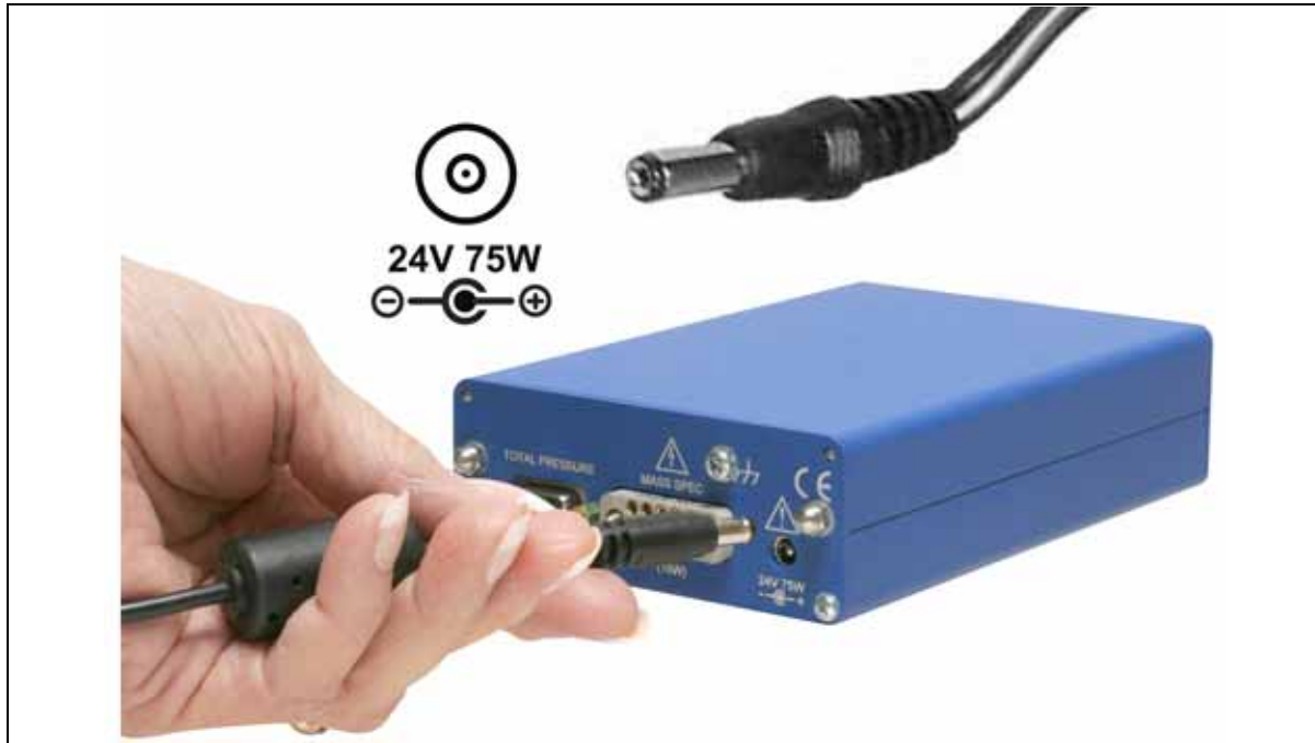
Figure 3-13 DC Power Plug
