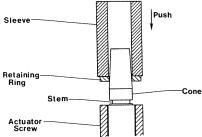
With the retaining ring "loaded," the sleeve piece is then pushed, expanding the ring on the cone and then down on to the stem until it springs into the groove.
