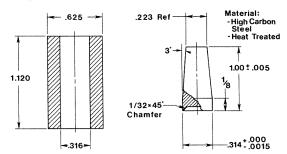
This tool is used as follows to expand the ring and push it on the stem.
