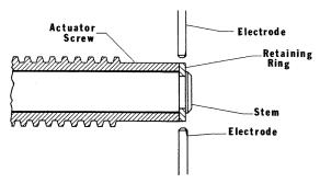
With the ring held between the electrodes, apply power so that the ring briefly glows a dull orange. Alternately, the heat may be applied for a longer time, making the ring brittle and easy to remove. After the ring has been heated, it is possible to grab the ring with pliers and spread it until it can be removed from the groove.
