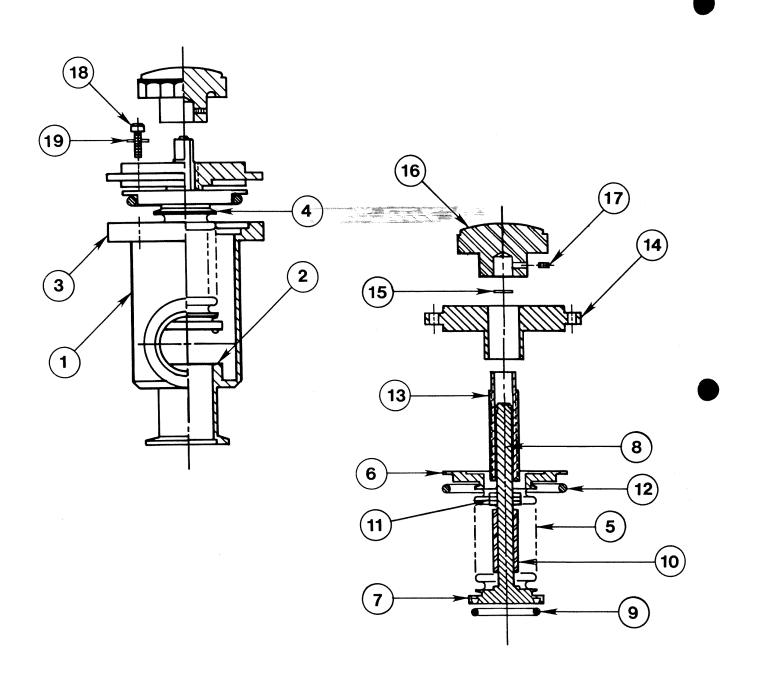
FIGURE 4 MANUAL ANGLE VALVE EXPLODED VIEW
