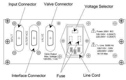
Figure 6: Rear Panel Controls
