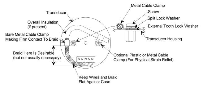
Figure 1: Preferred Method To Connect a Shielded Cable
