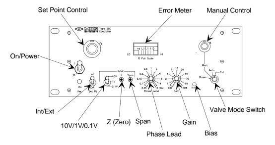
Figure 5: Front Panel Controls
